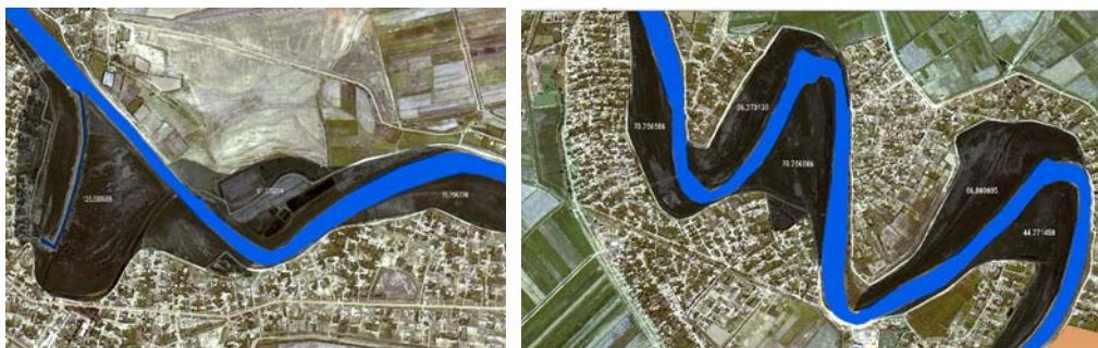
Fig . 1 Simulation of the risk of flooding from time-varying space information. Black contours of the forecast on the information of 2010 are superimposed on a picture of 2016.
